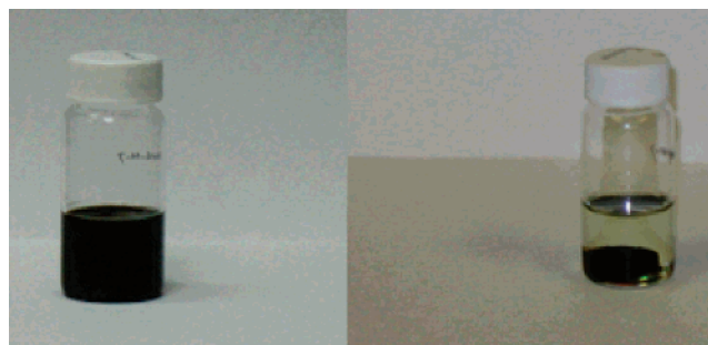
Figure 7. Dispersing and isolating the nanoparticle-supported catalyst.
